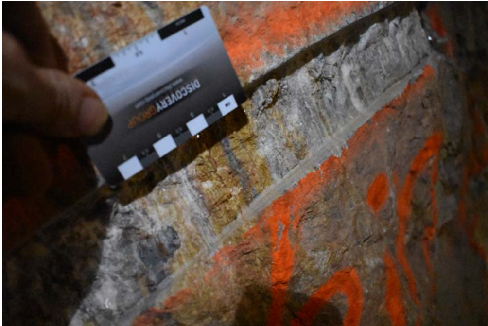
Figure 3 – Example of Underground Channel Sample
